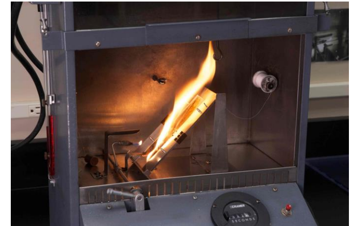
16 CFR Part 1610 Flammability Test Apparatus
